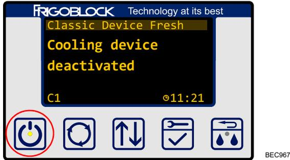
First the light inside the key will flash on and off and when the power-up sequence is complete the light will stay constantly on.
